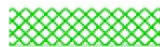
808 Prepared area Colour: upper green (PMS 354) Width of line 0.2 mm, distance between lines 0.8 mm, angle 45°
