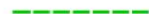
803 Track 0.8-1.2 m Colour: upper green (PMS 354) Width: 0.5 mm Length of a line 3 mm and distance between lines 0.5 mm
