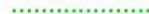
804 Track, slow 0.8-1 m Colour: upper green (PMS 354) Diameter of dots 0.7 mm and distance between dots 1.3 mm
